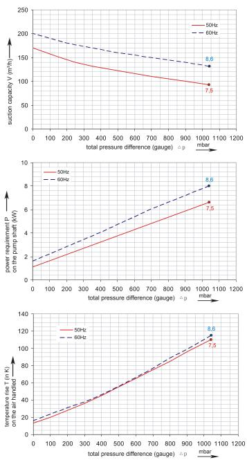
The performance curves are based on air at a temperature of 15 °C and an atmospheric pressure of 1013 mbar with a tolerance of +/- 10 %. The total pressure differences are valid for suction and ambient temperatures
